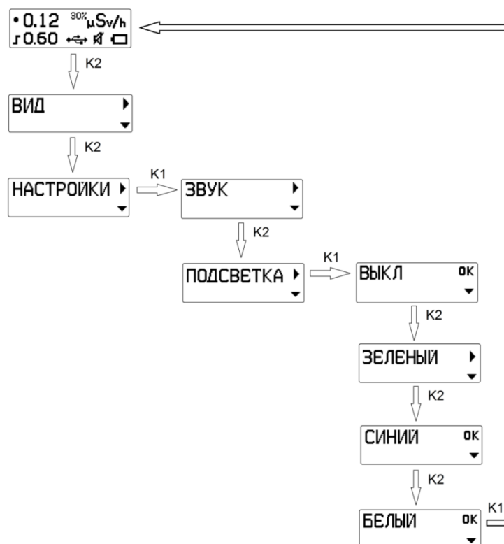
Picture 10 - Algorithm of switching on/off the display backlit
