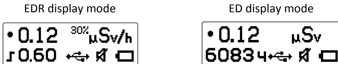
Picture 6 – The dosimeter display in EDR and ED display modes, in detail;
